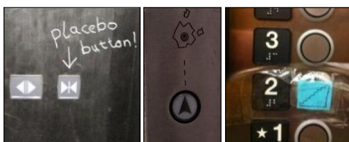
Figure 1: Three samples of dirty and damaged button panel
