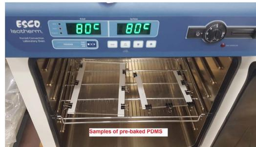
Fig. 2. Samples of pre-baked PDMS films interposed between PMMA glass plates prior to baking inside oven
