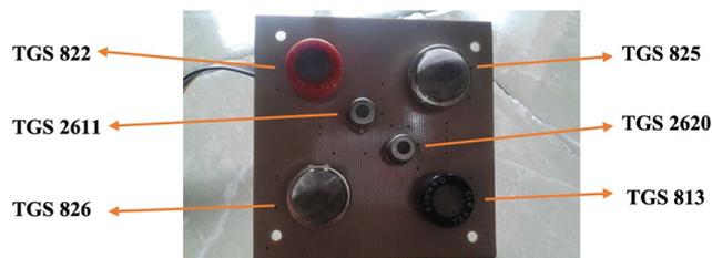
Fig 1. Array of Sensors
