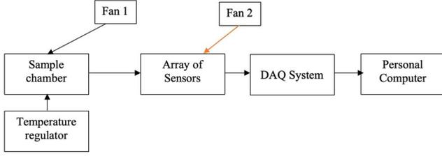
Fig 2. Block diagram of the e-nose used
