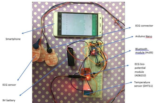
Fig. 4. Hardware setup for ECG device with temperature sensor
