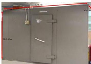
Figure 2. RF-shielded room for indoor measurement setup
