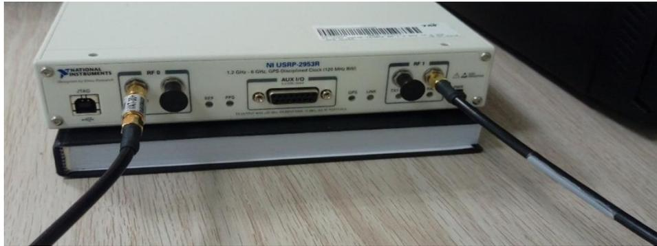
Figure 2. The wire is used to connect the transmitter and receiver for ideal case test
