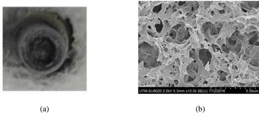
Figure 1. (a) Graphene slurry at the end of fiber ferrule, (b) FESEM image of Graphene slurry
