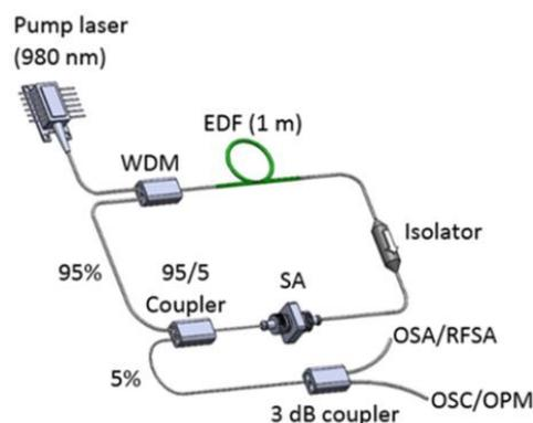
Figure 3. Integration of Graphene slurry based SA in fiber laser in ring cavity; OSA-optical spectrum analyzer, RFSA-Radio frequency spectrum analyzer, OSC-oscilloscope, OPM-optical power meter
