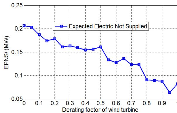
Figure 6. Reliability index EPNS of different derating factor of wind turbine
