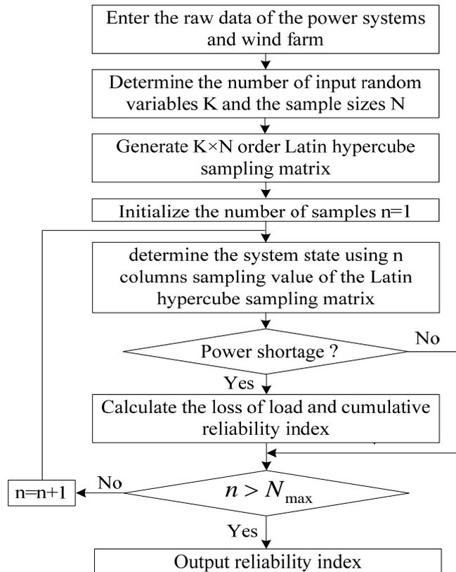
Figure 4. Process block diagram of reliability assessment
