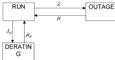
Figure 3. Wind turbine multi-state fault model
