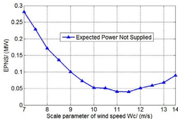
Figure 7. Reliability index EPNS of different scale parameter of wind speed
