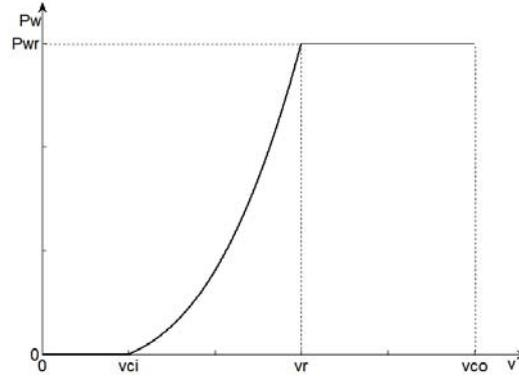
Figure 2. Wind turbine power curve
