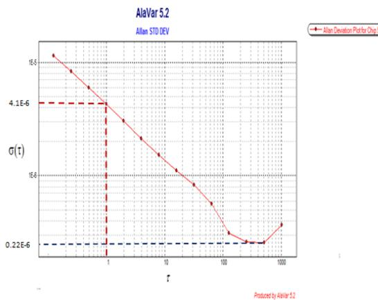
Figure 18. Allan deviation plot for Sandia 14 pin accelerometer
