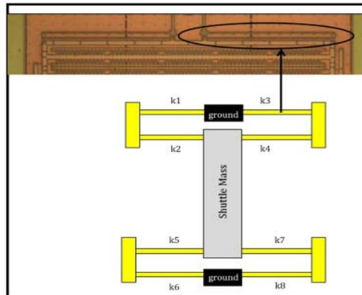
Figure 3. Sandia Capacitive MEMS accelerometer structure [6]
