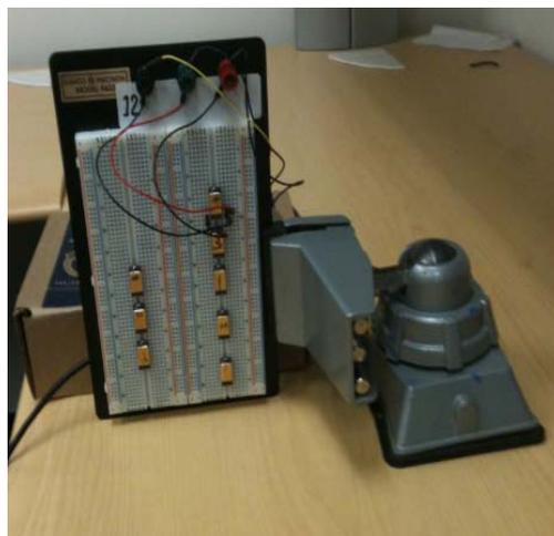
Figure 12. Test set up for Vibration test at 1g
