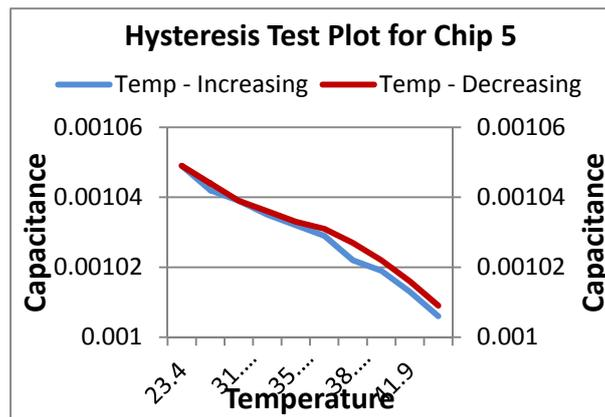
Figure 15. Hysteresis plot for Sandia 14 pin accelerometer
