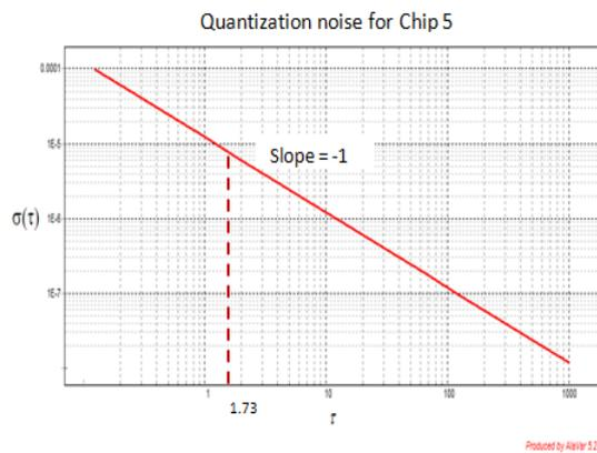
Figure 19. Quantization noise plot for Sandia 14 pin accelerometer
