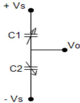
Figure 8. Circuit Model for Capacitive Voltage Divider [7]
