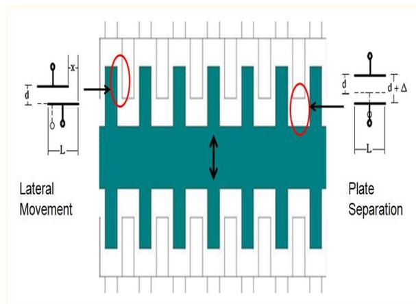
Figure 10. Electrode movements of comb-finger schematic [6]
