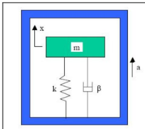
Figure 2. Sandia Capacitive MEMS accelerometer structure [6]
