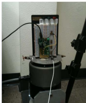
Figure 16. Test set up for Vibration test
