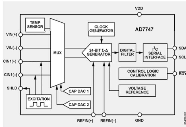
Figure 10. Functional block diagram of AD7747 board [8]
