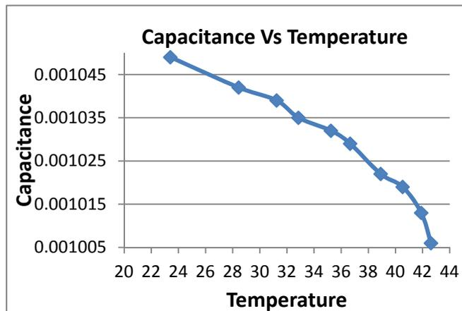
Figure 14. Thermal plot for Sandia 14 pin accelerometer
