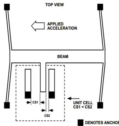
Figure 7. Movement of fingers when acceleration is applied [5]
