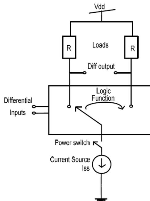
Figure 1. Basic MCML logic circuit
