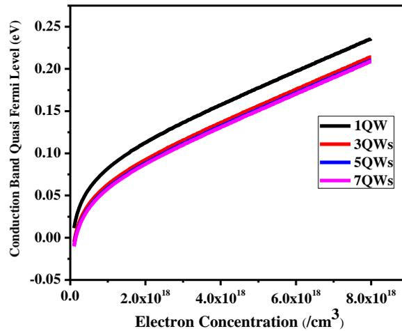
Figure 11. Quasi Fermi level in conduction band
