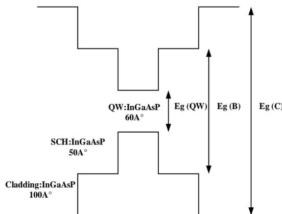
Figure 2. Schematic energy band structure of step index separate confinement SQW based InGaAsP/InP lasing nano-heterostructure
