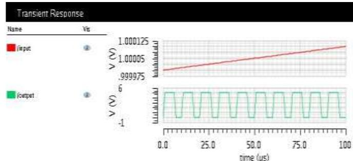
Figure 6. This diagram depicts the transient response graph of three stage Darlington feedback amplifier, which is obtained from the circuit diagram presented in Figure 4.
