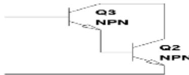
Figure 1. Basic circuit of single stage Darlington amplifier
